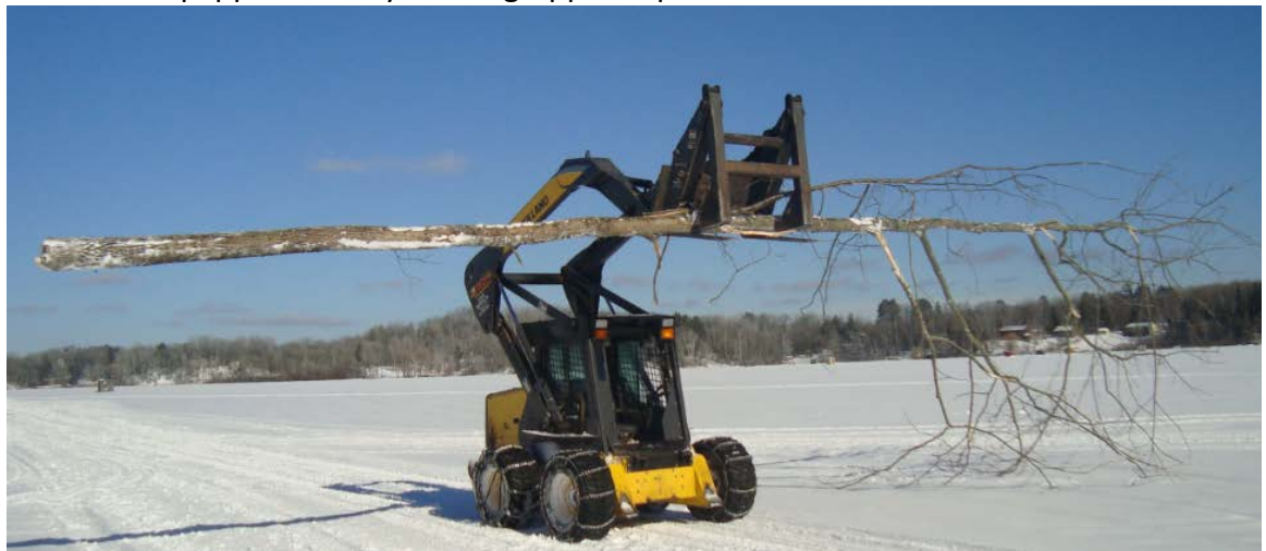
VII. Skid steer equipped with hydraulic grapple to place trees at site.
